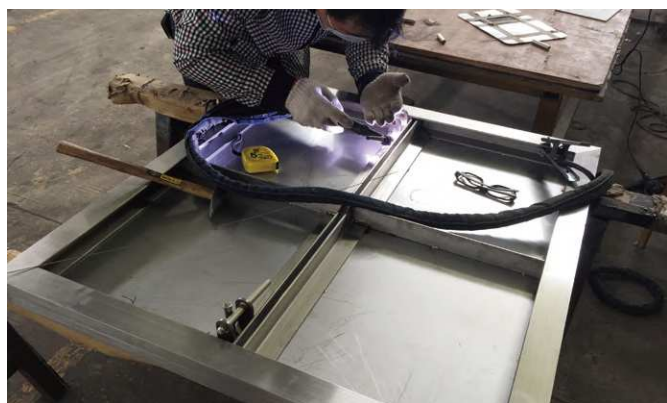
不銹鋼焊接 Stainless Steel Welding
