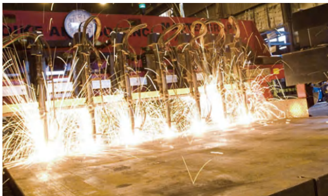
鋼材切割 Steel Cutting
