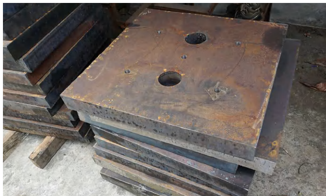
樁頭鋼板 Pile Head Steel Plate
