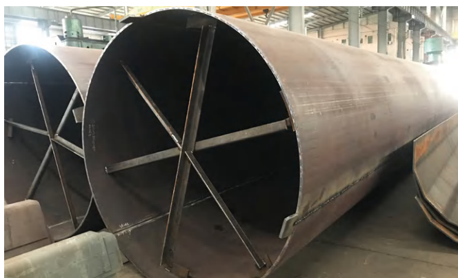
鑽探鋼管樁 Drilling Steel Pipe Pile
