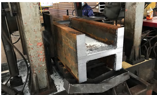
鋸床切割 Sawing Machine Cutting
