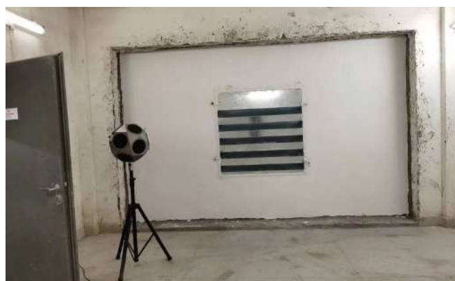
Fig. 2 - Louvers undergoing acoustic testing at the University of Auckland laboratory.
